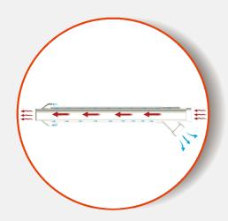
The concentric design cuts off the incoming fresh air and exhausts smoke. The preferred vertical roof terminal is not easily damaged, reduces the chance of absorbing pollutants, and sees less steam.
